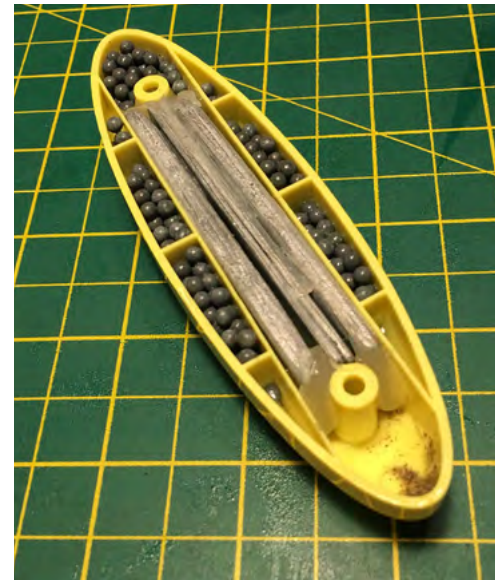
The saltwater weight module can be adjusted with lead shot
