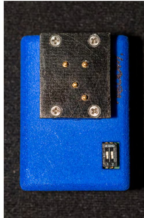
The underside of the TURTLE showing the DIP Switch in the bottom right corner that is set according to the make of strobe you are using.
