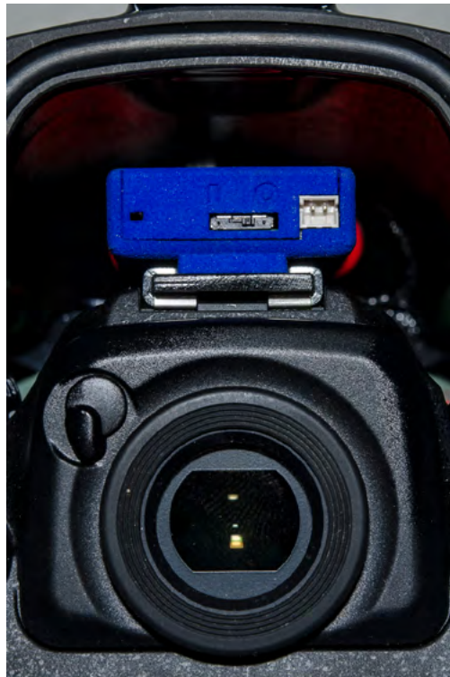
TRT Installed In Subal ND500 – The TRT easily fits into the Subal ND500
