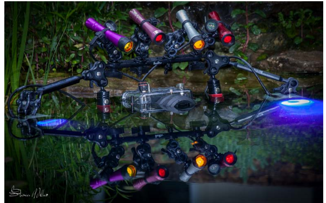
Fluorescence luminance setup. The colored Gammas above are constantly on for color and for seeing around you. When the flash goes off the light emitted is blue as it passes through a dichroic filter, the first step in Fluorescence shooting.
