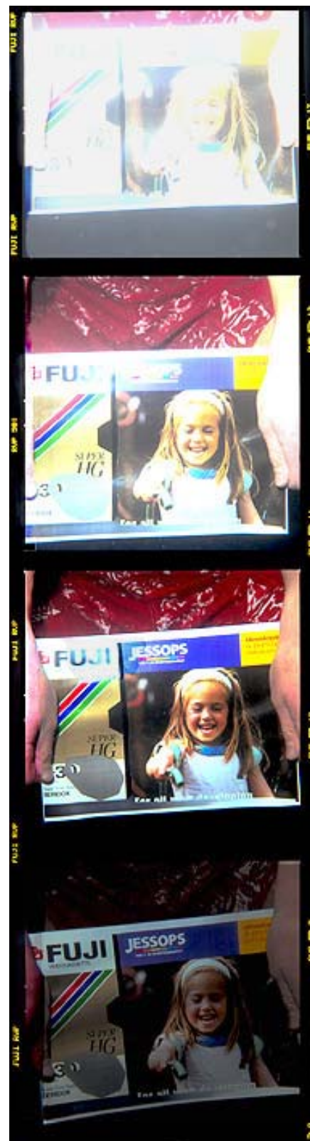
An example of a calibration film, Southampton, UK. Hasselblad 500C/M with Zeiss 80mm and 0.5 Proxar close-up lens. Sea and Sea YS 120 flash on FULL power. All exposures at 1/250th on Fuji Velvia. Apertures from top f8, f11, f16, f22, with f16 producing the best exposure.
