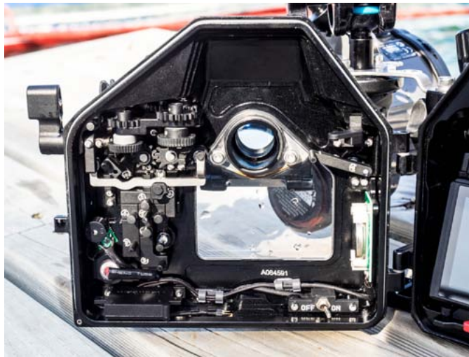
Nauticam rear door with vacuum system electronics and upper left auto focus lock control.
