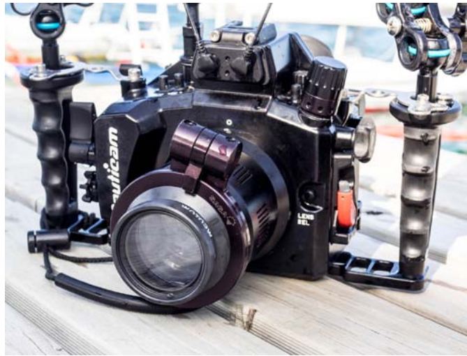
New Nauticam front port lock (red) and the vacuum valve, with the new grips.
