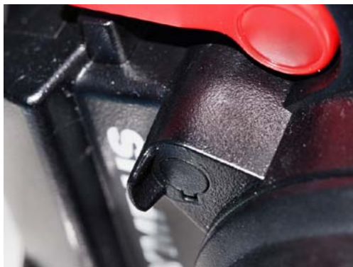
The offending port cover that needs to be removed to use mini-domes
