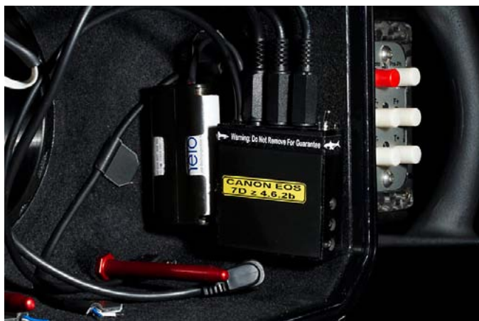
The ‘heart’ of the housing: The USB electronic control unit plus batteries.
