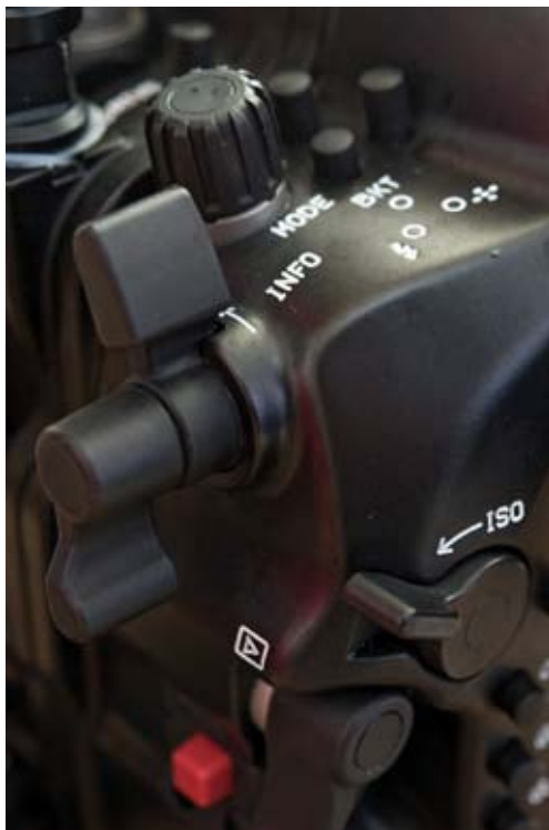
Details of levers for Image Review, INFO and ISO, conveniently positioned by Nauticam to fall under the right thumb, rather than having to push buttons.
