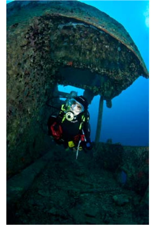
Thistlegorm forward port walkway 2011 – the same location this year has very little coral growth left and stanchions have been torn away on the port gunwale by mooring lines. Nikon D300, Subal ND2, 10-17mm FE zoom, Inon Z240 flash guns, ISO 200 f11 1/80
