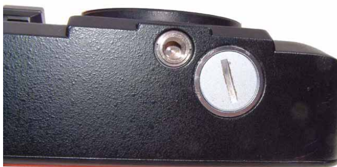
(Above) Newer models have a chromed ring fitted around the battery compartment. Older models (left) don't have this ring
