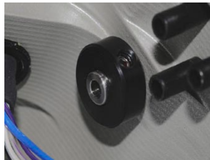
Replacement of shutter mode release/lock control with new shorter control (i.e. for selecting single frame, continuous)
