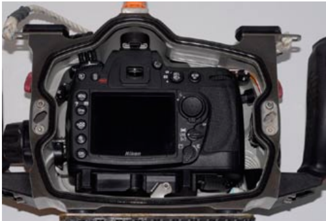
D300 mounted in the ND20 housing.
