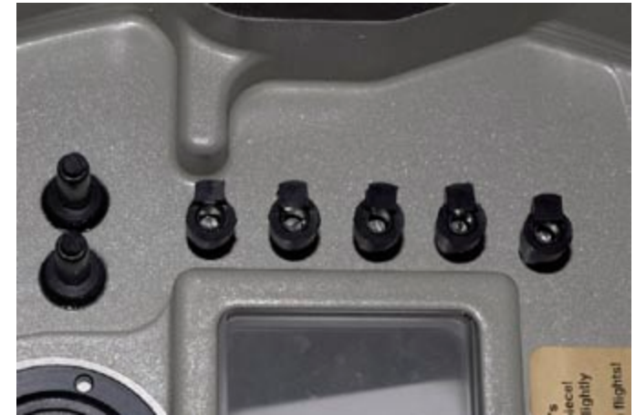
Push on extension pegs for buttons on left hand side of D300 review screen.
