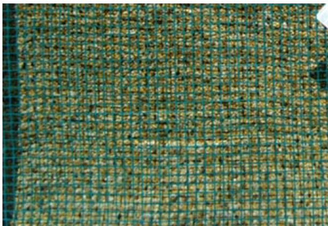
Seacam recommended 35mm extension with Superdome. No dioptre. Quarter crop, corner bottom left. 12-24mm at f8. 1/125th ISO 100
