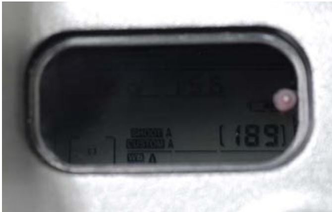
Sloping window for top LCD frequently throws shadow across part of the LCD.
