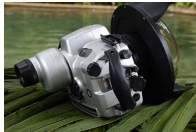
Starboard side of Seacam showing S180 viewfinder with Superdome and shutter, command dial, AF/AE lock and sub-command dial controls.
