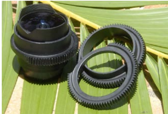
Home-made gears for the 10.5 fisheye and Sigma 15mm fisheye.
