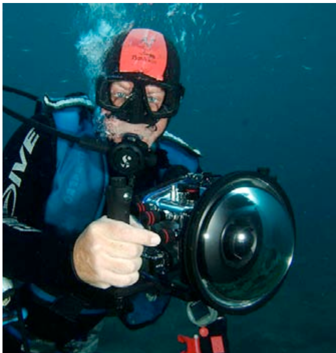
The large dome port worked well with the Nikon 10.5mm fisheye producing no flare but the test conditions were a slightly overcast day.
