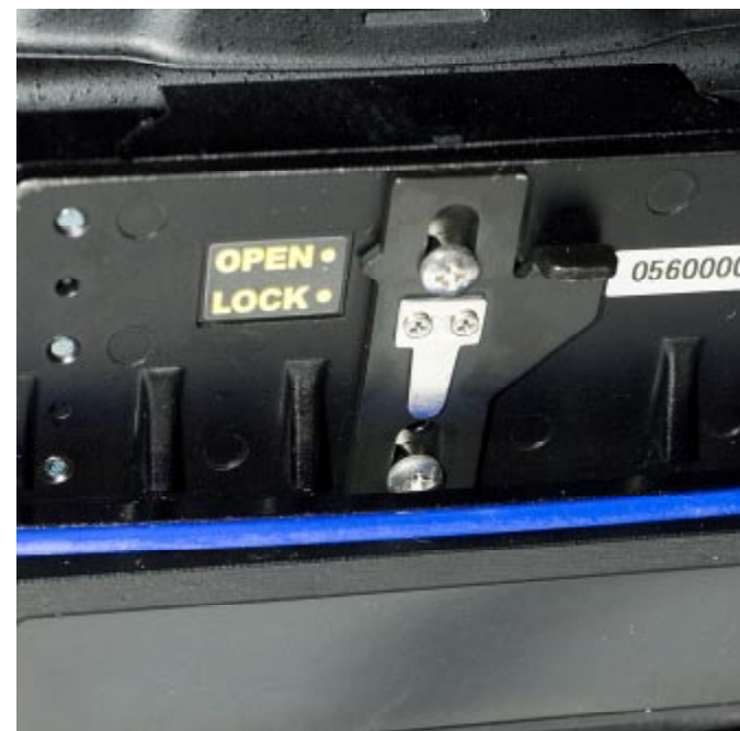
A locking mechanism located underneath the hotshoe can be used to prevent accidental removal of the port.
