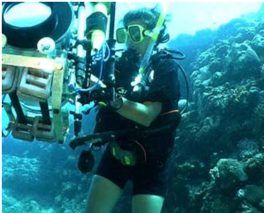
Dolly in mid water, shows weights beneath camera on rails - depth 8m.
