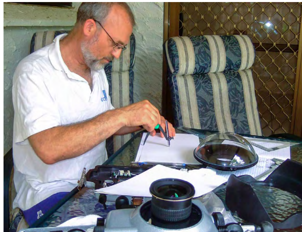
Darryl Torckler making a pattern to measure the radius of one of his dome ports
