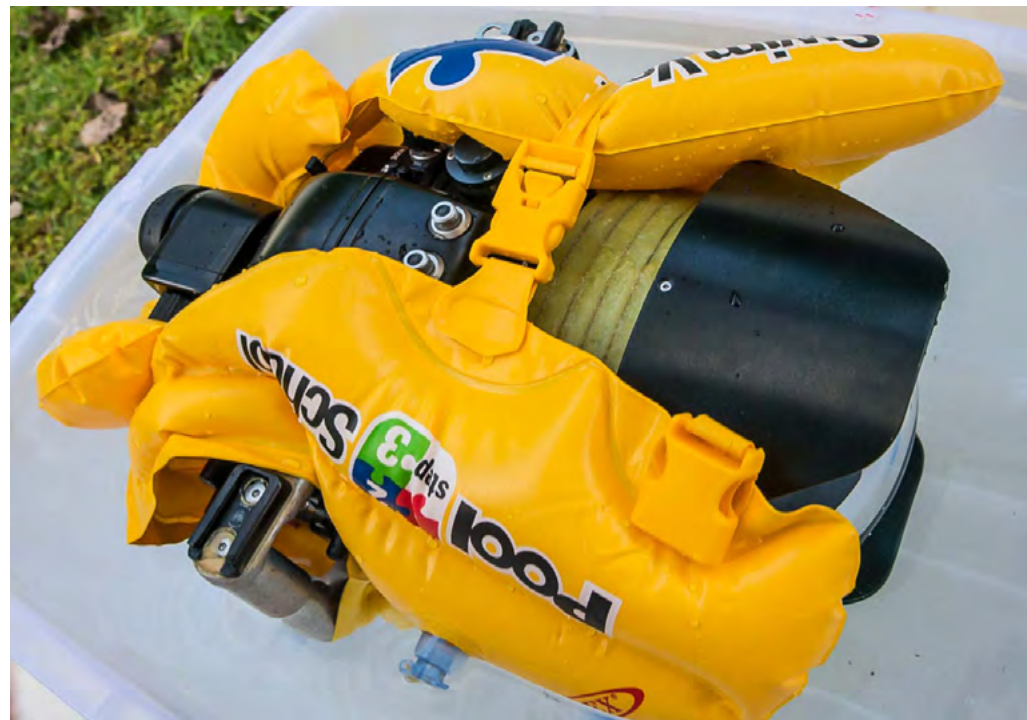
A child's life jacket can be used to float the housing at precisely the right depth. Here my D800 housing also has a foam buoyancy collar around the port extension
