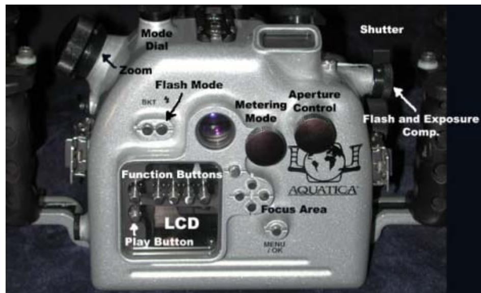
A view of the housing back showing the layout and function of the controls.
