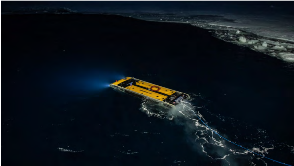
The multi-role, 3000m rated, Saab Sabertooth is the world's only roaming and hovering robot that can operate in both fully autonomous and tethered modes, enabling fully flexible dual operations from a single platform fitted with cameras, sonars and tooling.
