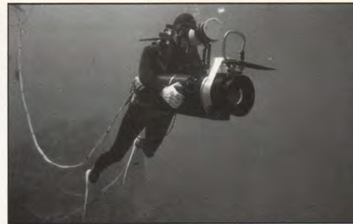
(Left) Peter and his "Scoones Cam" venture out. The "flag" over the lens provides shade and minimises flare. The umbilical carries communication and video signals to the surface.
