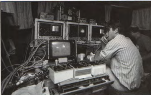
(Above) Peter Scoones looks through the monitor to check the camera port for any signs of blemishes which may appear on the screen and lower the quality of presentation.
