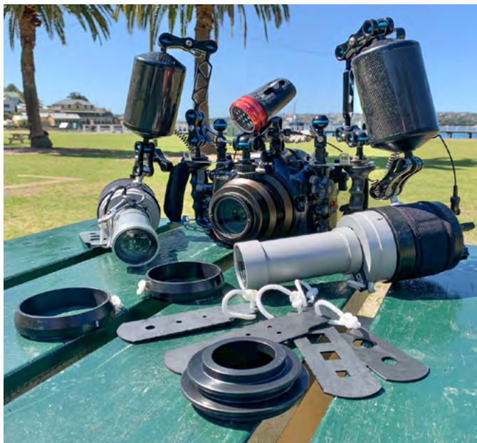
A pair of Retra Flash Pros with LSDs, bumpers and neoprene covers, mounted on our Nauticam NA-D500 housing. In the foreground, the regular reduction rings, macro reduction rings and masks sets for the LSD snoot
