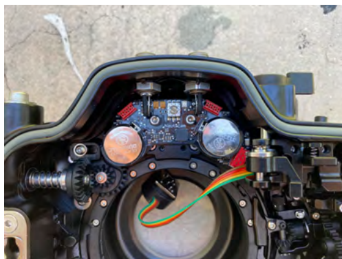
Inside rear view of the NA-Z50 housing with the Nauticam optical strobe trigger board installed.
