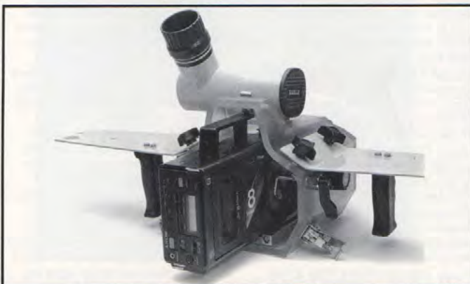
Above: The rear of the housing is held in place by three large stainless steel catches with snap-in safety locks. Tape cassettes can be loaded and removed without having to remove the camera from the housing but a battery change means total removal.
