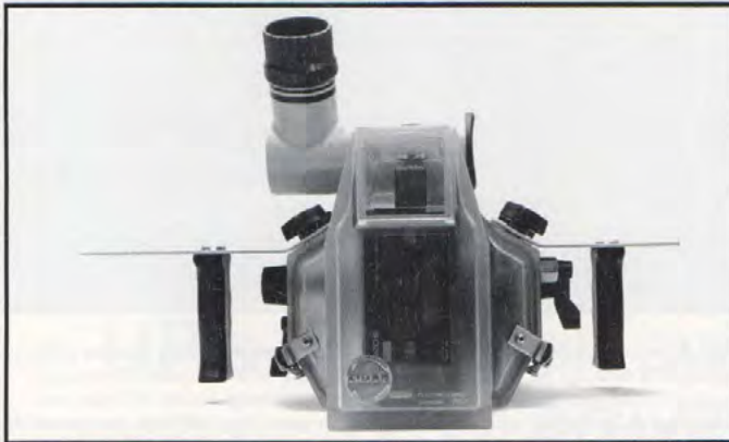
Above: The LCD panel can be viewed through the rear of the housing to see the tape counter, battery indicator and recording status. It would be possible to fit other controls here to rewind and replay the tape underwater.
